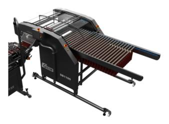
These machines have a buffer chain for sticks and can load the sausages on the D732 unattended. Depending on type and
