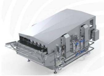
The cured sausage moisturizing unit for high performance is composed by a completely automatic water management system it allows to reuse the water by continuous filtering through a double filter. Automatic filling system by electrovalves, water level and temperature management.
